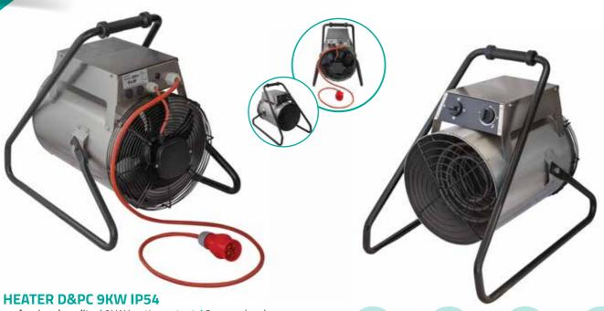
professional quality / 9kW heating output / 2 power levels + ventilator mode / adjustable thermostat up to 80°C / air flow 1700m<sup>3</sup>/h / power supply 3x400V/50Hz / power cord 1,5m / 5 pin male plug
